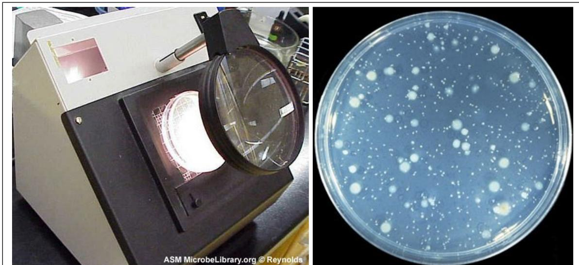
**Figure 1. Bacterial Colony Counter and Pour Plate.** The bacterial colony counter (left image) is used with pour plates (right image) to help determine cell numbers in a sample. Note that two types of colonies arise in and on the pour plate. The larger round colonies form on the surface of the medium, whereas the small ovoid colonies are growing within the agar medium.
