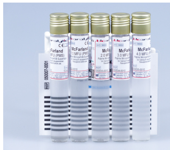
Figure 2. Wickerham card and various McFarland standards of turbidity.
