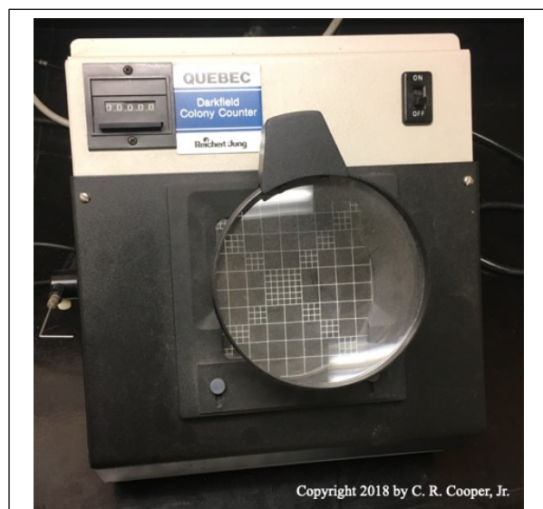
Figure 7. Colony Counter. The colony counter can be used with spread or pour plates to count the number of colonies.
