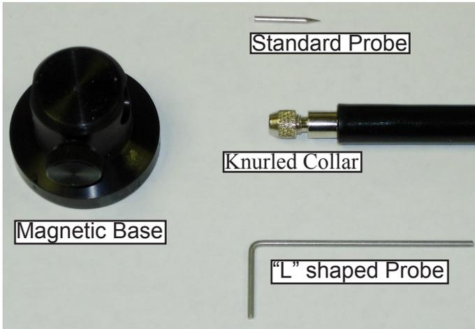
1. Loosen knurled collar and remove the standard probe.
