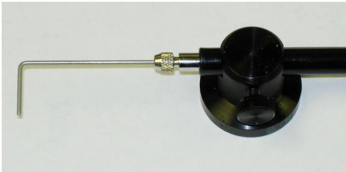
2. Insert the probe handle into the hole on the magnetic base and tighten it in place.
